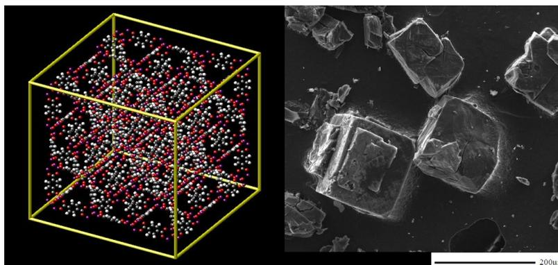
Fig. 1 MOF-5 Structure (Left), and SEM of MOF-5 (Right)
