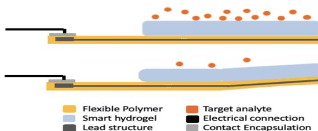
Figure 2: The sensing approach in which fentanyl changes result in bending of a multilayer hydrogel/polymide structure, thereby producing an electrical signal.
