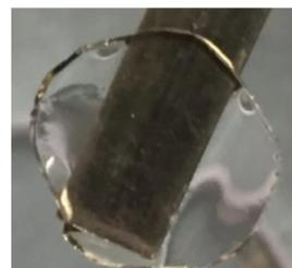
Figure 1: A transparent hydrogel on a metal surface
