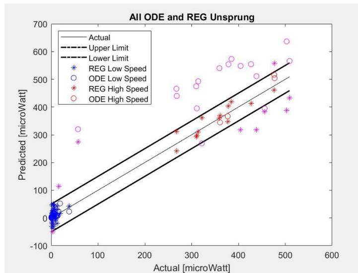
**Figure 2: Unsprung Device, Predicted vs. Actual Power Output**
