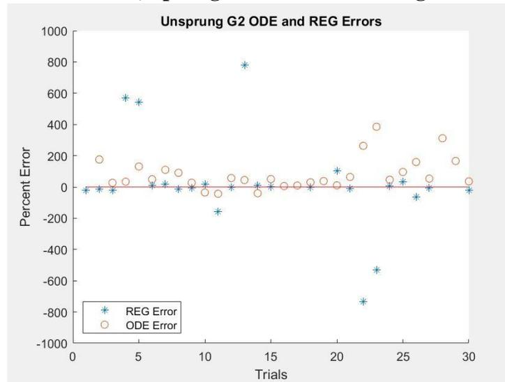
**Figure 4: Generation 2, Unsprung Device ODE and Regression Error Plot**
