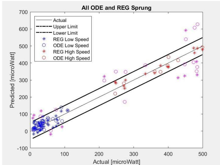
**Figure 1: Sprung Device, Predicted vs. Actual Power Output**
