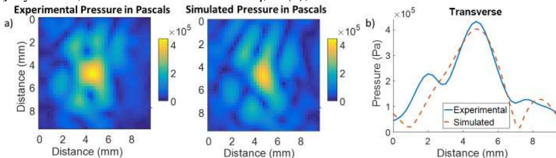
FIGURE 1: Comparison of hydrophone measurement and HAS simulation in (a) transverse plane and (b) transverse peak pressure trace after propagating through a heterogeneous phantom.
