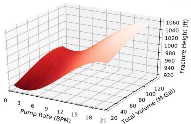
**Fig 2.** Fracture height response surface for pump rate vs. total pump volume
