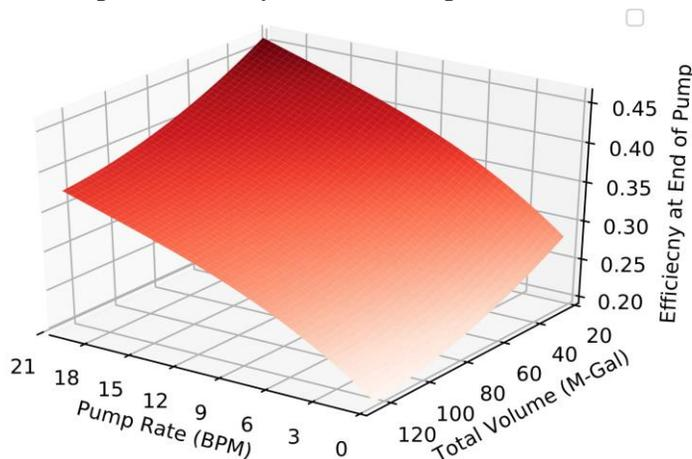
**Fig 1.** Efficiency response surface for pump rate vs. total pump volume
