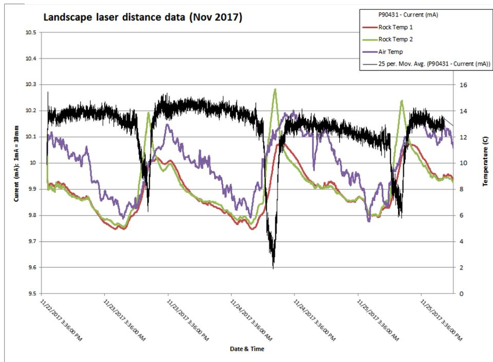
Figure 2 – Laser distance data (black) paired with air (purple) and rock (red and green) temperature data measured between November 22<sup>nd</sup> and 25<sup>th</sup>, 2017 at Landscape Arch.
