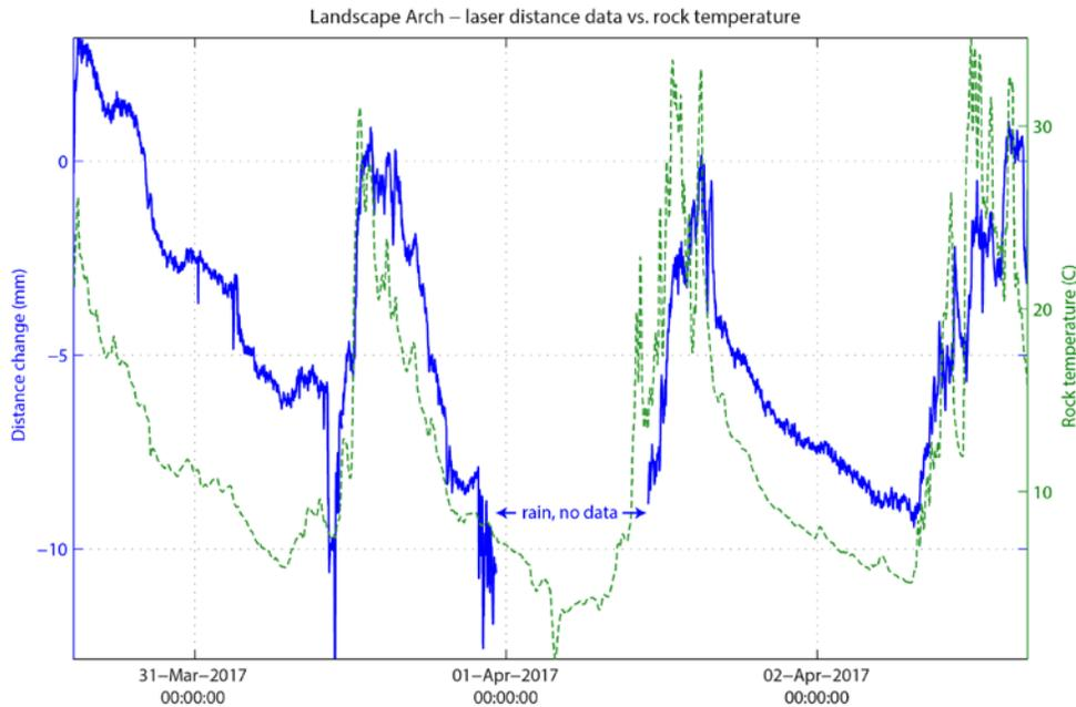
Figure 1 – Laser distance data (blue) paired with rock temperature data (green) measured between March 31<sup>st</sup> and April 2<sup>nd</sup>, 2017 at Landscape Arch.
